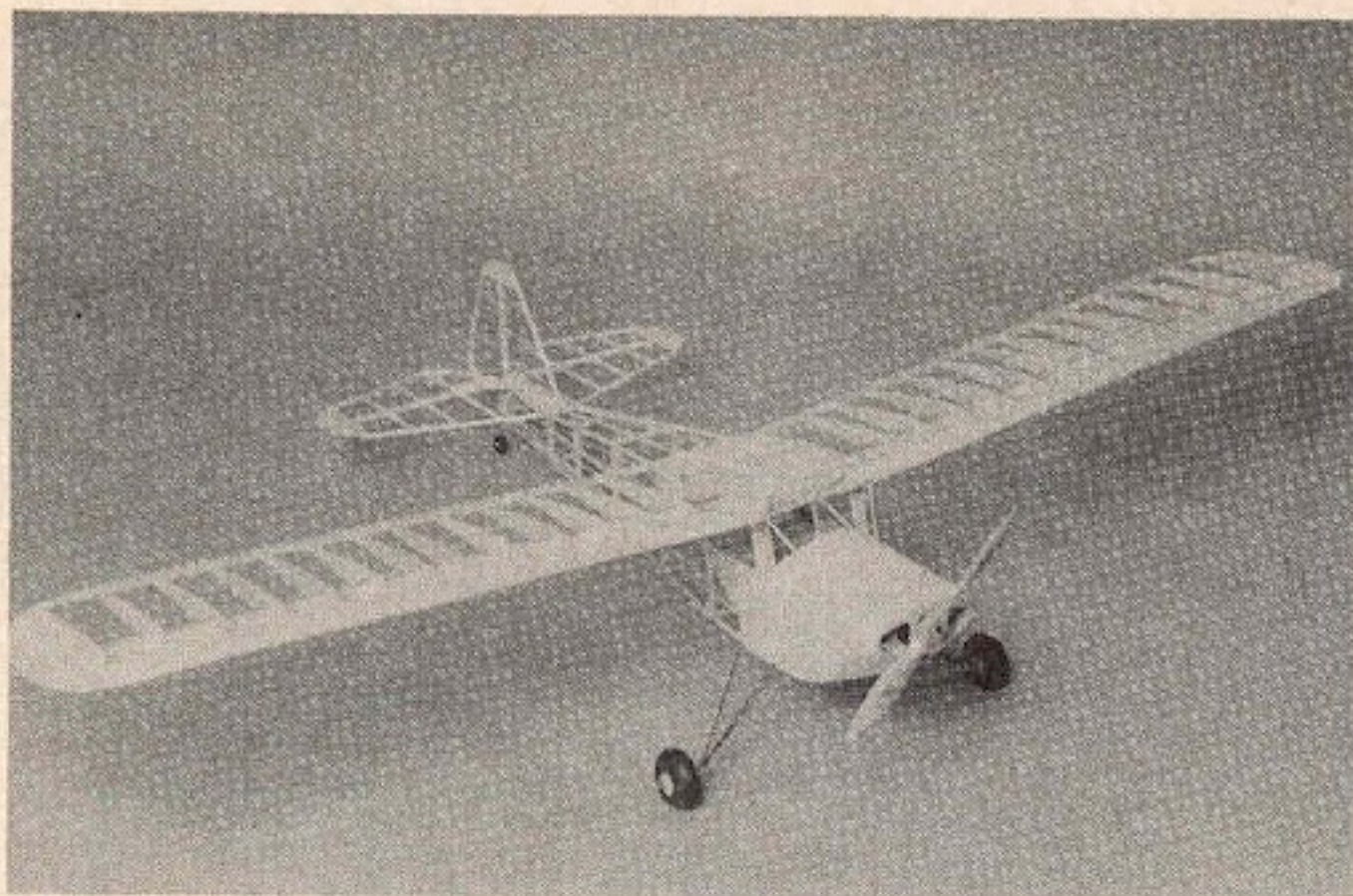
Uncovered electric powered Taylorcraft sports lightweight stick construction.
