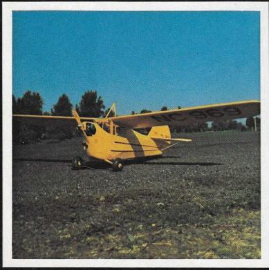
A magnificent classic from the Golden Age of Aviation, the 1935 Aeronca C3 Master is the last version of what was probably the first true ultralight plane commercially produced in the United States. The "Airknocker" was actually not much more than a powered glider with its high aspect ratio wing and two cylinder, 36 horsepower engine - - - -
