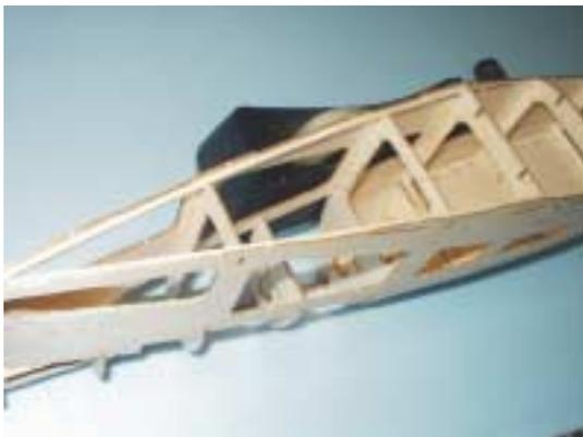
Cut some 3/32 square sticks and glue along the fuselage bottom being sure that they fit into the notches in the bottom of the formers. Now glue the bottom in place.
