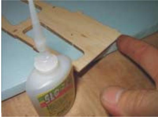
Place the two fuselage sides on top of each other lining them up EXACTLY. Now take some slow CA and smear it across the rear of the fuselage taking care not to get any glue in between the two sides. When dry this will form a "hinge" allowing you to now open the sides up in perfect alignment.
