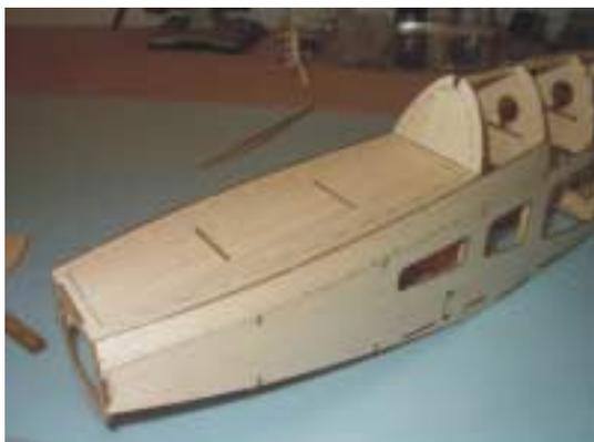
Next glue former F4B in place as well as the upper fuselage sides. Make sure the sides are oriented correctly with the bigger end at the rear.
