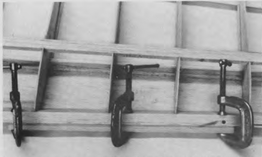
Glue on the bottom 1/16" sheeting. I used clamps and a block of wood to hold the sheeting to the leading edge while gluing.
