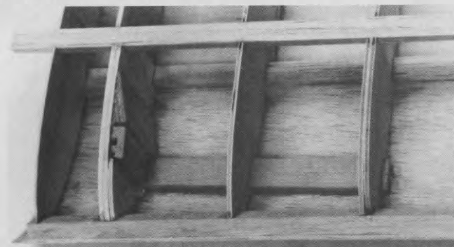
Cut away the sheeting for the landing gear blocks and glue them in place. Add W-28, the vertical gear block, and the 1" trailing edge stock rear brace.
