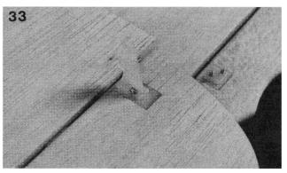
may now be started. Proper alignment of the bulkheads to the location marks on the bottom is important as is the squareness. Bulkhead F-3 is shown in the photo with the forward servo mounting rail glued in place.
