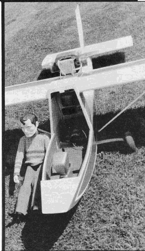
ABOVE: Wing and stab surfaces are removable. RIGHT: Photo showing interior. Notice fuel tank location. No problem drawing the fuel using just muffler pressure. Homemade muffler to simulate opposing twin. BELOW: The pilot is a must to complete the package.
