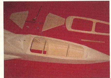
The forward section of the fuselage showing the canopy/hatch as well as the canard control surfaces.
