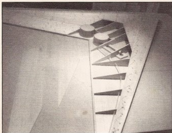
LEFT: Top sheeting is being applied. Notice the nylon tubing for antenna. RIGHT: Elevon torque rods installed. Notice pencil marking on fuselage bottom sheeting.
