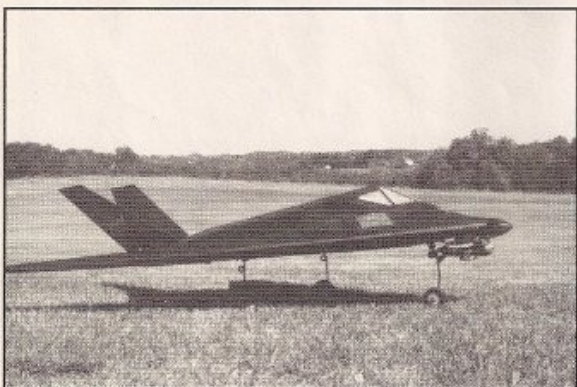
LEFT: The finished model. The nose gear is slightly longer for test flight. RIGHT: A nose high landing and touchdown on the main gear.
