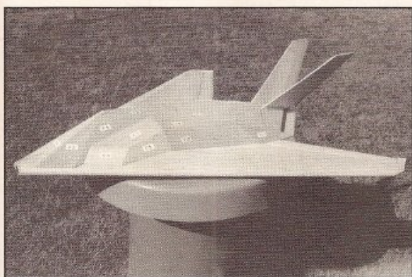
The built-up model with the fuselage panels clearly labeled.
