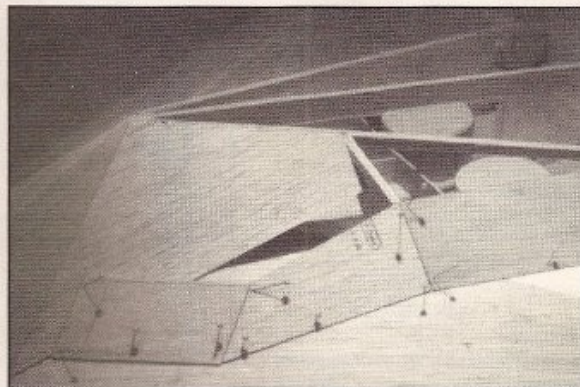
LEFT: Exhaust slot structure. Note the reference line on L2B for E4. RIGHT: Fuselage panels being glued in place. Install one panel at a time, on each side.
