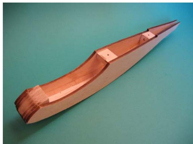
Now trim the rear slot between sidewalls to get the 6 mm gap in order to accept rear fuselage part later (the boom assembly).
