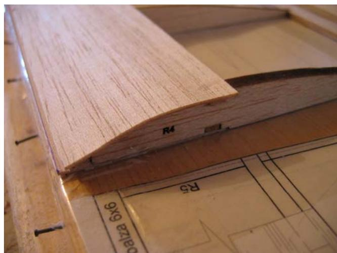
In order to attain pressure in the gluing areas, you can use simple but efficient method. Put some short nails on the both sides of the assembly board as shown on photo above. Well, you should do nailing before starting of assembly of the wing.
