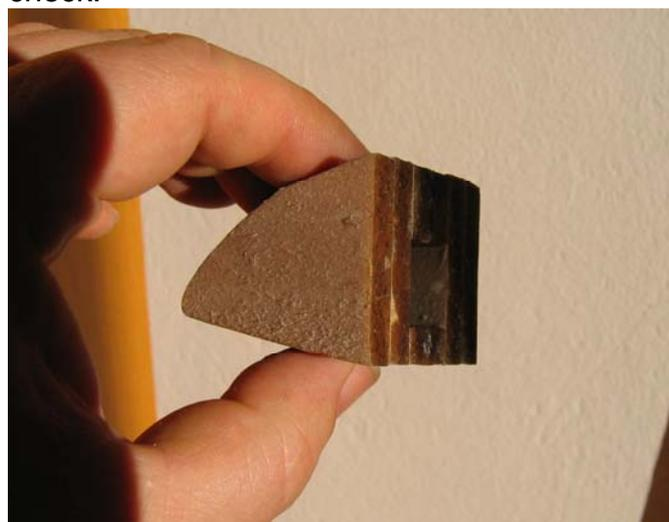
Now it is time to find a proper location and glue that nose block on to laminated lower part of the fuselage.
