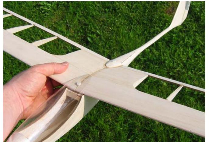
Now you can cover the model with your preferred covering film and at your desire for the overall outlook of the model. But you can also use Guppy »standard« design as shown on plans and this assembly manual.
