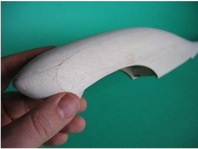
If you choose electric powered Guppy, then you should cut the nose block at location where diameter of nose is the same as your prop spinner (30mm). Look at the plans and allow for some »down trust«. Drill a hole in the nose block. Use oval rasp to file the hole to dimension slightly over 27mm, to accept SPEED 400 motor. Now bolt the first plywood former on the motor and test fit that on the nose block. Correct if necessary and when O.K., glue nose former to the fuselage nose block.
