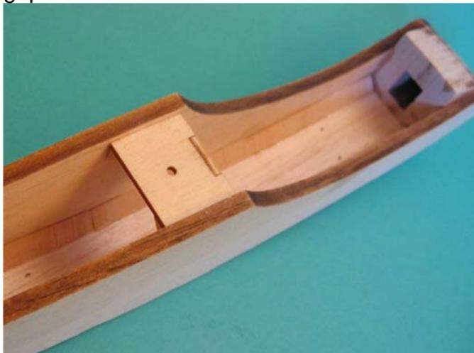
protrude on the top of the fin about 5 mm, and glue it to place using CA glue. After that glue opposite fin covering; also balsa plank 1 mm thick.
