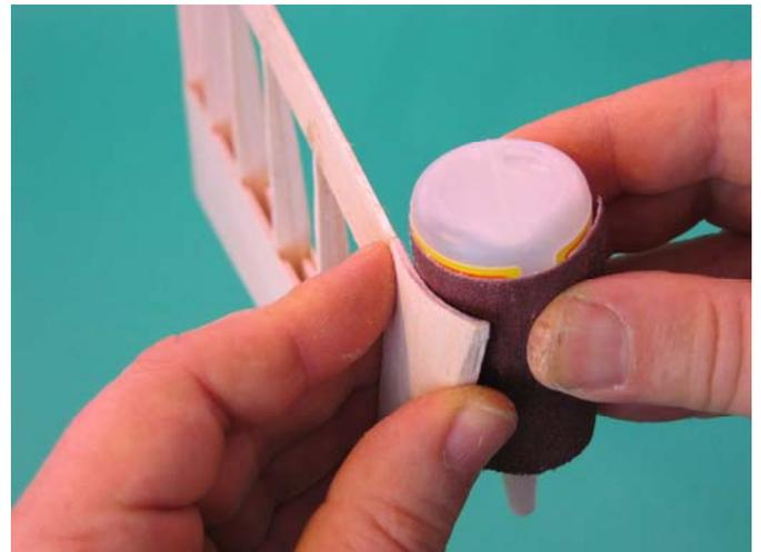
You can sand the wing tip shape with sandpaper wrapped around oval object (CA glue bottle in case shown on picture above)
