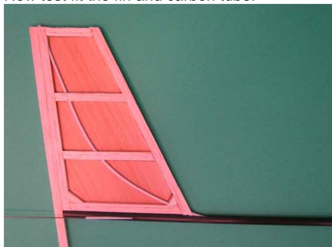
Now we will assemble the balsa parts around that carbon tube.
