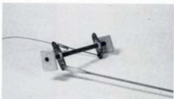
Titler bar for elevator. Pushrod from servo rotates bar, and four cables (only one shown) go through fuselage skin to elevator horns.
