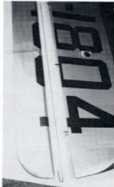
Hinging system for ailerons... provides neat and scale-like closed gap, also more efficient.
