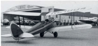
This photo, and the one at the top, were taken soon after completion of the Moth, in 1960. Sprung tailkid is later replaced by steerable wheel. Functional exhaust from Forster .99.
