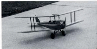
Another just-completed photo. Former .30 was unable to get the plane off of a slow-cut grass field . . . was later replaced by Fox .50 that powered very first "Big John".
