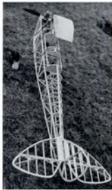
Fuselage and tail framework. Fuselage sheathed with 3/32 balsa. Nylon covering over all.
