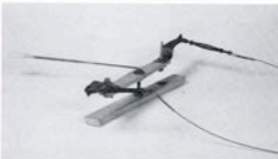
Sled-type rudder bar. Ends stick through slots in fuselage side and cables are on outside. Pushrod from servo operates bar.
