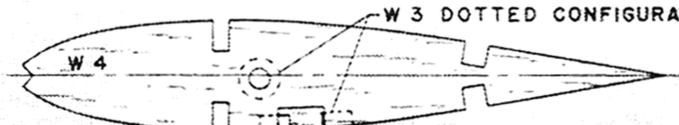
W 5 SAME AS W 4 LESS L. G. NOTCH & HALF OF SPAR NOTCH
