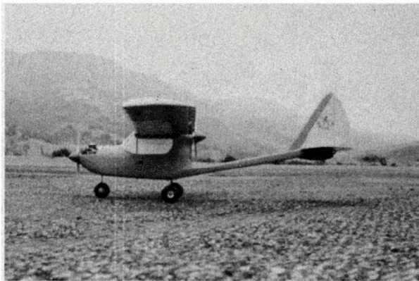
The twin waiting to do its thing. You can see slight negative angle of attack of wing in this position.
