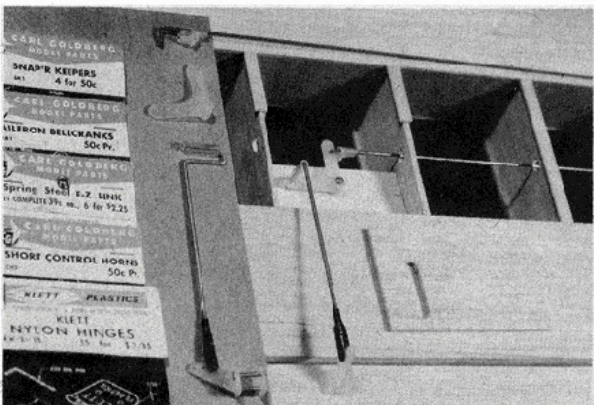
Aileron control parts and installation. Pushrod from bellcrank to horn can be removed for wing covering and reinstalled.
