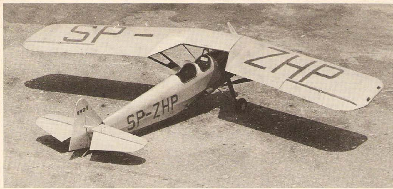
A view of our SP-ZHP. The sharply swept back wing effectively moves the C.G. back so that short nose is not a problem as it often is.
