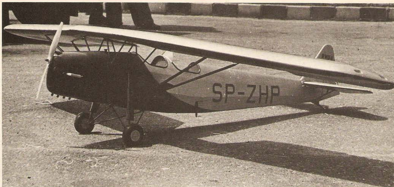
This view of our Polish two-oler makes it look droopy winged, but it really isn't, though it doesn't have any dihedral at all, builds easily.
