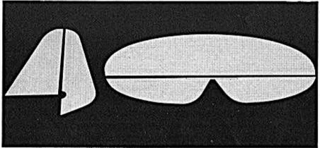
Cut out the tall parts from 3/32" balsa. Join the elevator halves with 1/8" dowel.
