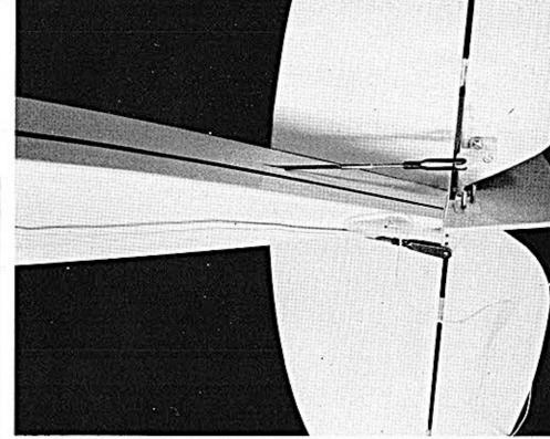
Pushrods and control horns. Loop the radio antenna through two holes drilled in the Goldberg wing skid used for the tall skid.
