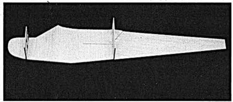
Glue the firewall and bulkhead B to one of the fuselage sides.
