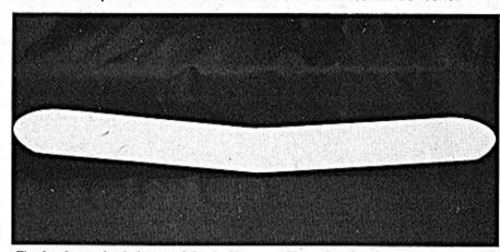
The Ace foam wing halves are joined with epoxy. Shape the wing tips using the template cut from the plan. Cover the wing with EconoKote or other low temperature covering.
