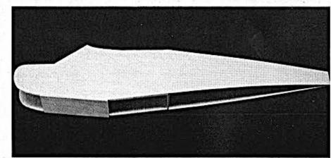
Glue on plywood bottom C, and the landing gear doubler D, and install the two 4-40 landing gear blind nuts. Pull the tail together and glue.
