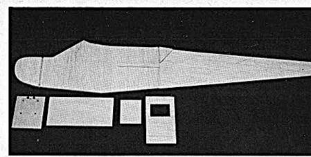
Make the fuselage sides from 3/32" balsa with 3/32" vertical grain balsa doublers using the template cut from the plan as a guide. Drill the firewall for the fuel lines and install the blind nuts for the motor mount. Cut out C and D from 3/32" plywood.
