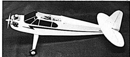
Cover the model with EconoKote and decorate with black MonoKote trim. Add the dummy balsa engine. Hinge the rudder and elevator. Install the landing gear, engine and radio. Glue on the tail group.
