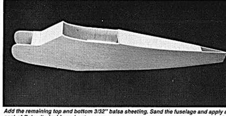
Add the remaining top and bottom 3/32" balsa sheeting. Sand the fuselage and apply a coat of Balsarite inside and out.
