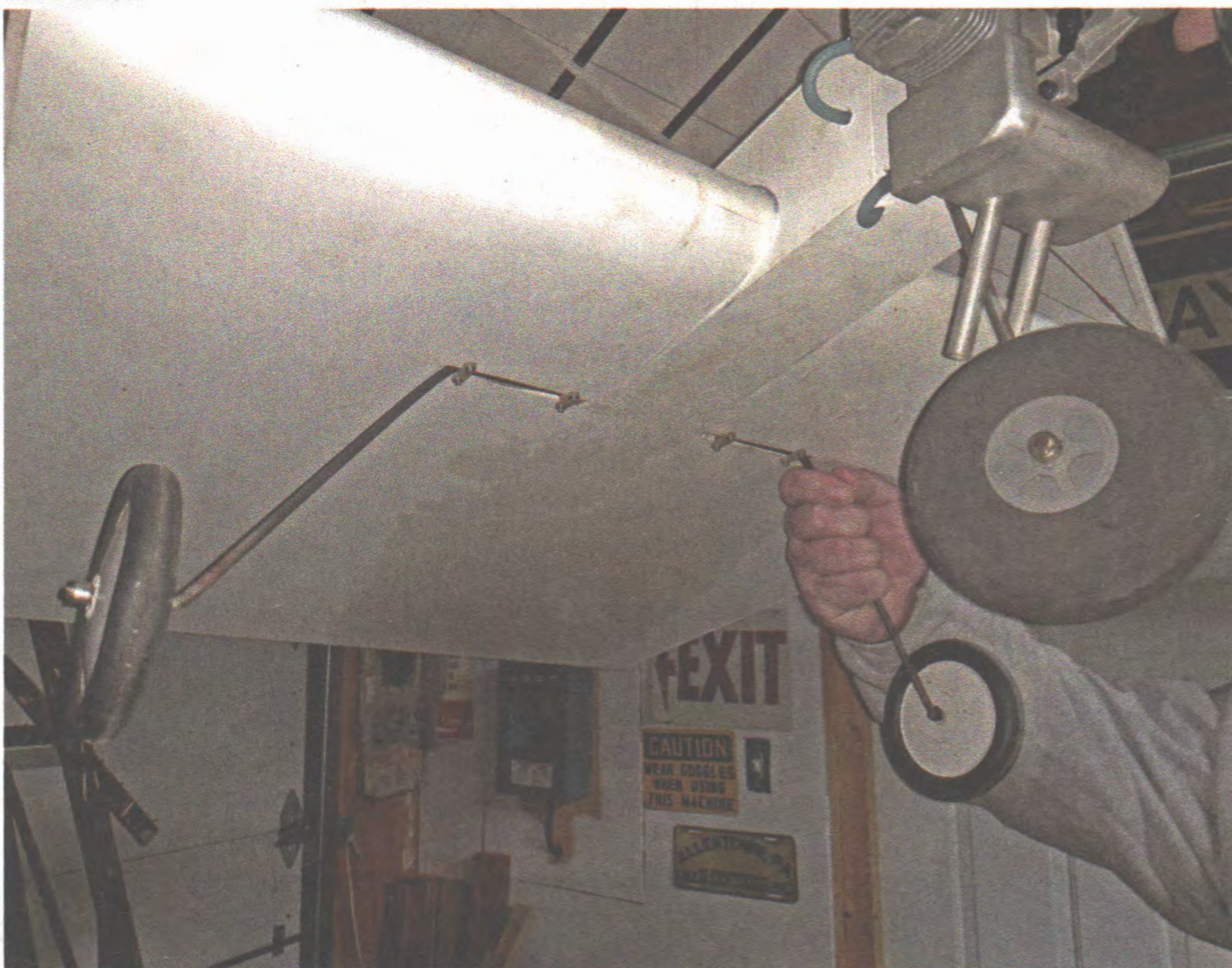
The tricycle landing gear is normal and set up for a slightly nose-down attitude while the model is at rest.
