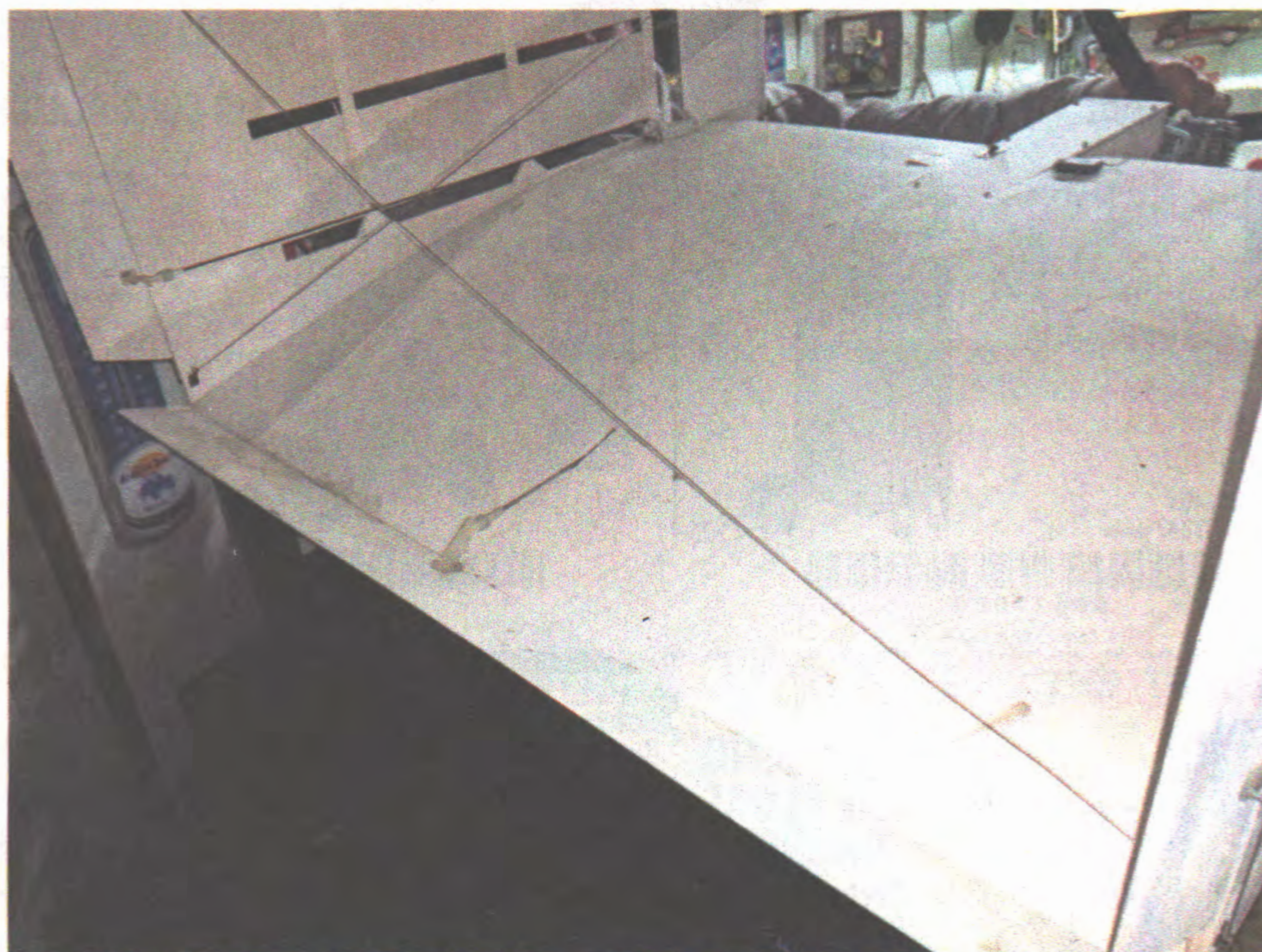
This rear view shows off the elevator and control linkage. The twin rudders have a servo for each control surface.
