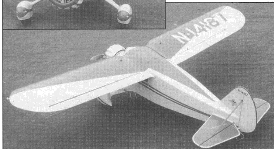
N14187 paint details. Each color, including pin-striping, is masked separately.
