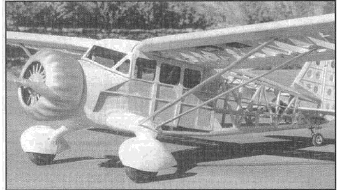
Ready for covering. Entire model, including side windows, will be covered with clear MonoKote and painted. Mask the windows to keep them clear.
