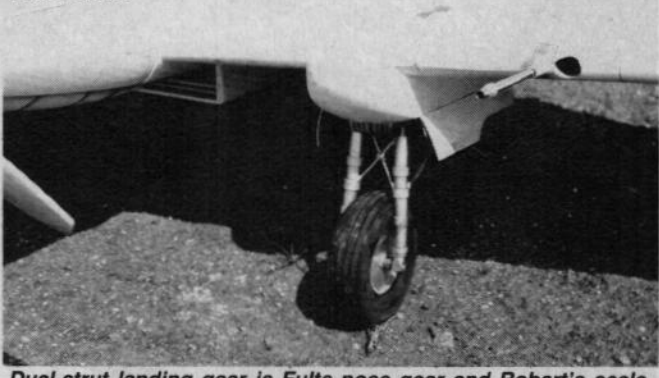
Dual-strut landing gear is Fults nose gear and Robart's scale wheels. Cannon barrel is removable, breakaway soft aluminum tube.
