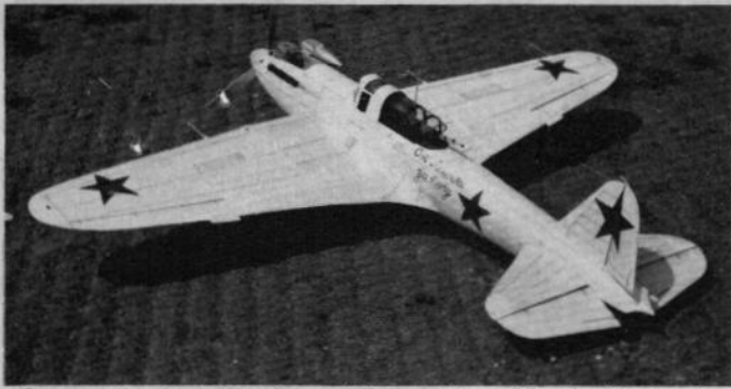
Stormovik's high-lift wing and large tail combined with slender, long fuselage are good proportions for a scale model. Stable flight, excellent ground-handling.
