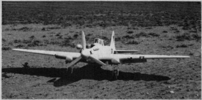
Panzer's view of oncoming Stormovik. Low, wide-stance landing gear designed for rough Russian airfields makes for good ground-handling. Flaps are in lowered position.
