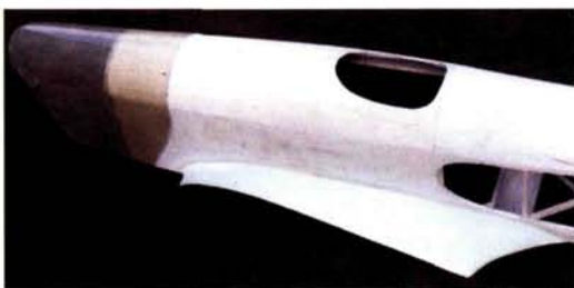
The tops of the fillets are formed of foam and covered with fiberglass cloth and resin.
