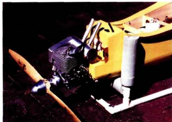
I used a Zenoah G-62 and a Slimline muffler to power my Sparrowhawk. To install and remove the narrow engine cowl, you must remove the carb from the engine.
