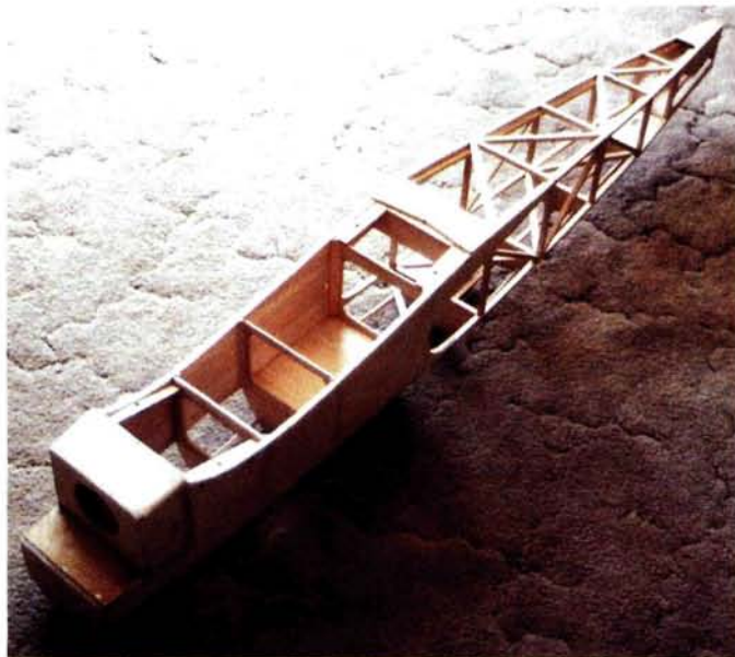
The fuselage is a light, strong structure. Note the staggered firewall; it provides room for the engine and muffler in its narrow cowl.
