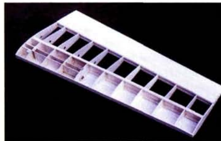
Top: each wing panel is built separately and then joined to form the completed wing. Above: here, the leading-edge sheeting and the leading edge have yet to be installed.
