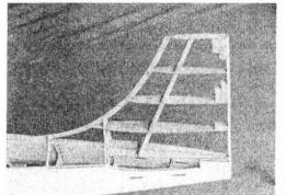
the pattern on the plan and soak with 50/50 water and ammonia mix if required. Fit it so the front edge sits in the middle of F-13. Cover one side and trim the front to follow the airfoil contour. Let the second side overlap this. Trim this to form a sharp leading edge. It will be final shaped later.
