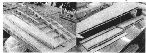
hard wood joiners and WJ-1 fit properly. Cover the top of the wing from the center of the main spar to rear 1/8"x 1/4" spar. Do this with the wing on the plan and washout strip in place. I use "Sig-Bond" or "Titebond" on the ribs and rear spar. Put the pre-joined sheet in place and tack it in a few spots to the main spar with thin CA glue, Zap. Pile about 4 inches of model magazines on the wing. Before the
