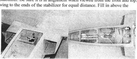
and screw the aluminum heat shield and aluminum engine cover in place. Set control throws as shown. Balance 7" back from the leading edge at the fuselage. Place the receiver battery and weight as required in the nose to obtain this.
