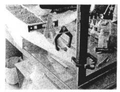
Cover the fin from the spars to the tail post with 3/32" balsa. Let the covering overhang the tail post by about 1/8". Be sure the fin remains in alignment. Now cover the front of the fin with 3/32" soft balsa. Use
