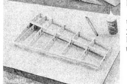
Remove the assembly from the plan and add the bottom spar. Sand the top of the trailing and leading edges to conform to the ribs. Do not remove the rib legs yet. Make 3/32" balsa sheets that will cover from the center of the spar to the leading edge and to the trailing edge plus 1/4" extra. Run the wood grain along the leading and trailing edges.
