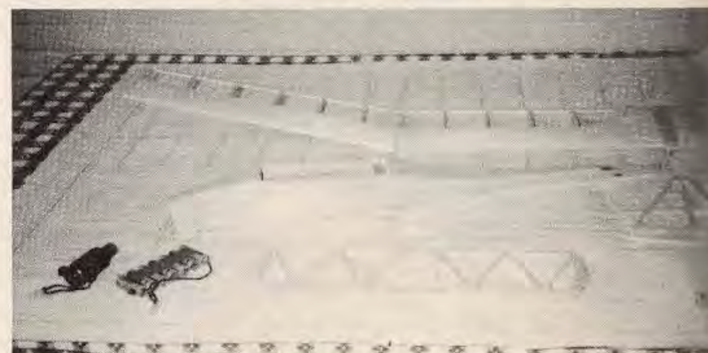
Completed components of the Electraglide II ready to cover.
