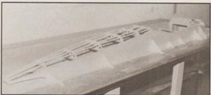
No fuselage jig is required since the fuselage can be built accurately over the plan.
