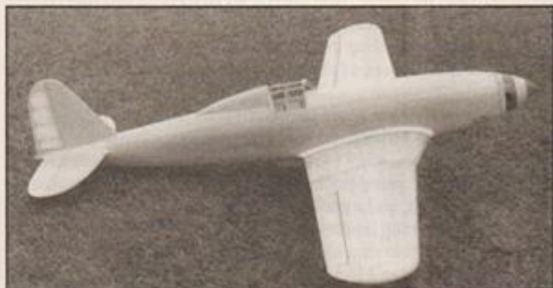
Long tail moment, evident here, helps the Fiat to groove like a pattern plane.
