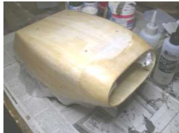
The entire radiator can be covered with one piece of \frac{3}{4} oz glass cloth.
