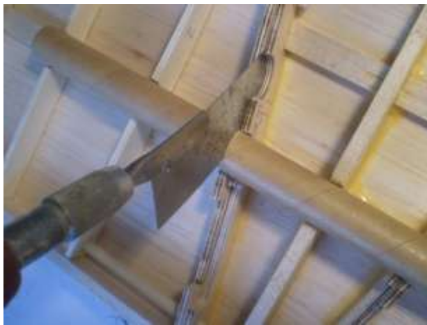
Cut the tube with a backless razor saw.
