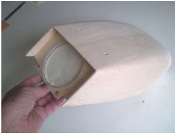
Completed radiator, ready for glassing.
