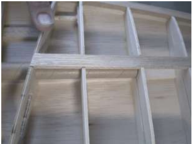
Fit, but don't attach the lower half (not yet sheeted).
