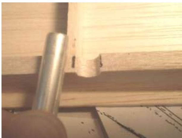
File a half hole at all hinge locations, top and bottom. Glue the upper and lower stab halves together. Add a 1/2" strip of 1/16" sheeting to the trailing edge of the lower half, leaving a 1/8" overhang as was done in the upper half. This will help alignment when fitting the elevators in the next step while leaving the interior accessible.
