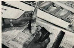
Using thinner to remove spar pieces from rib. Cap strips removed with model knife.
