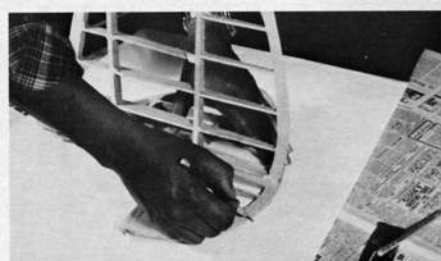
After removing half of stab, rudder could be laid down flat to trace outline. Everything was traced directly from model parts.
