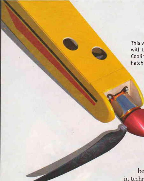
This view of the nose section shows the motor with the folding propeller bolted in place. Cooling air-inlet holes are used in the removable hatch, which uses a spring-loaded latch.
