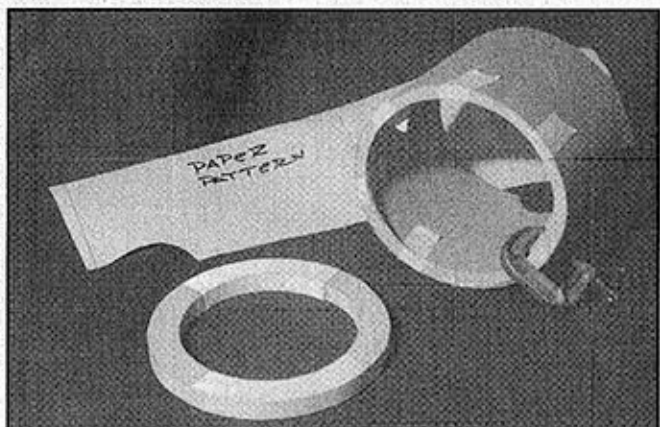
Cowl 1/32" ply being glued to 1/8" ply former. 1/2" balsa nose fairing ring in foreground to be glued on next and sanded to shape.
