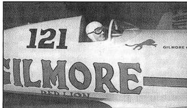
Gotta have a pilot. Cockpit trim is ironed-on after canopy is glued in place.
