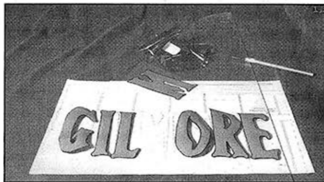
Cut each letter using a pattern Xeroxed from the plan. Bond to black MonoKote and trim for approximately 1/16" pinstripe. Align letters on glass over pattern under glass with tabs of masking tape. Apply Frisket paper strip across center of letters to hold letters in alignment for application.
