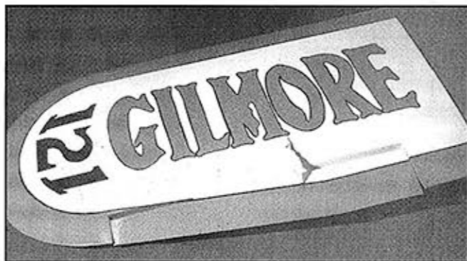
Graphics detail showing all MonoKote trim. Aileron is hinged at top surface with MonoKote for airtight seal. Pinstriping is sandwiched between main and trim color covering using lowest heat needed to activate the adhesive.
