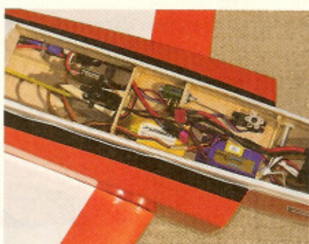
With the main hatch cover removed, you have plenty of access to the radio system and battery.
