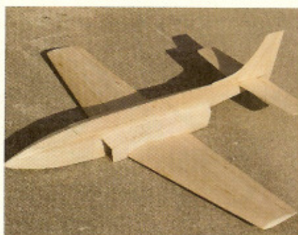
Here's the completed airframe ready for covering and the addition of the form canopy available from the author.
