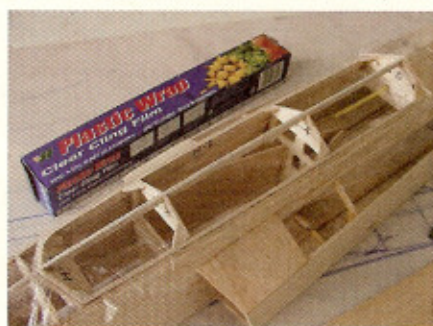
To make the removable hatch, cover the hatch opening with plastic wrap and build the cover in place on the fuselage. The wrap prevents the hatch cover from being glued to the fuselage.
