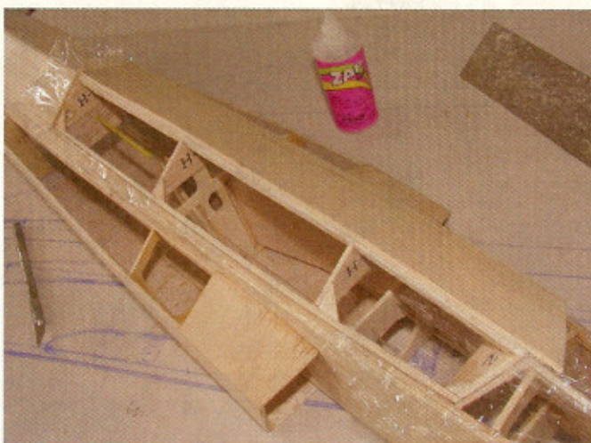
Here is the fuselage sheeting being glued into place.
